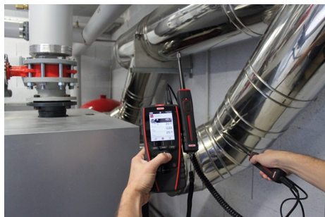
Hygrometry and air velocity measurement
