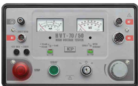
HVT-70/50I control panel
