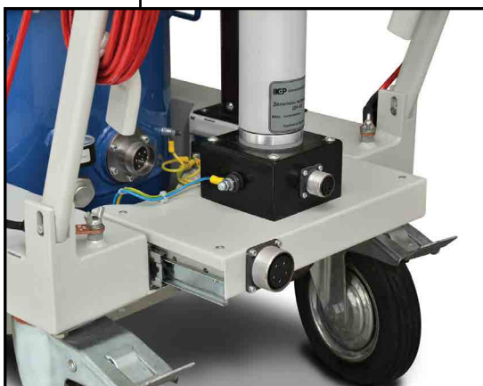
The connectors for control unit connection
