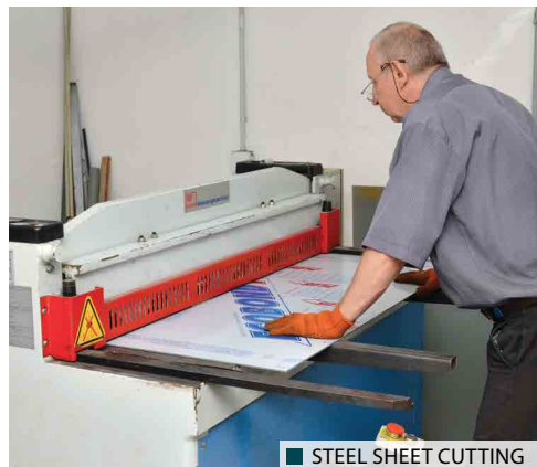
STEEL SHEET CUTTING
