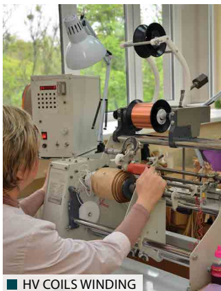
HV COILS WINDING
