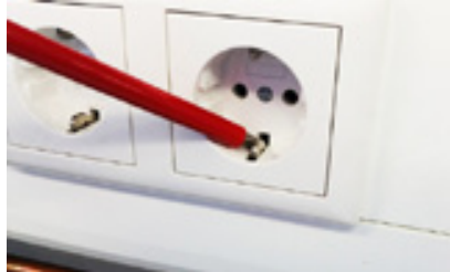
Self-test with the help of the PE contact of a socket
