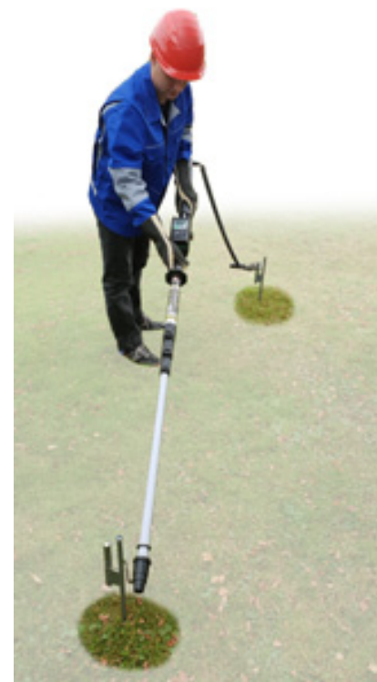
Check earth by second earth spike
