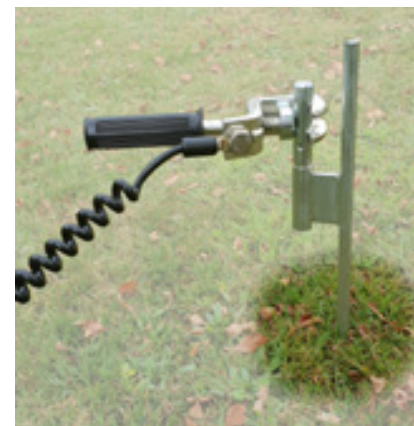
Earth connection with earthing spike and universal clamp
