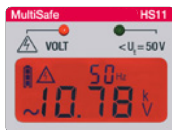
Colour change of the display at voltage
