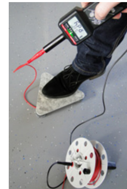
Check the conductivity of ESD floors
