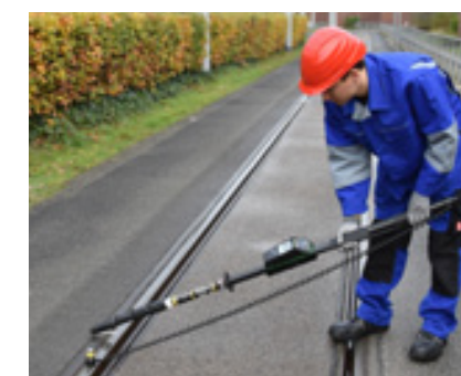
Complete self-test of device function and contact with the rail within seconds
