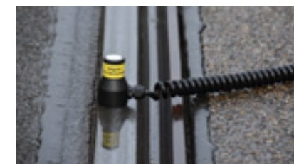
MultiSafe TT 1-MA with magnet
