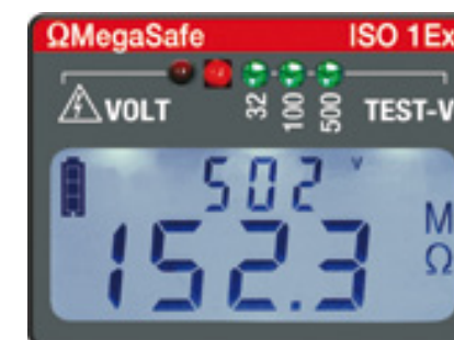
Check the conductivity of ESD floors
