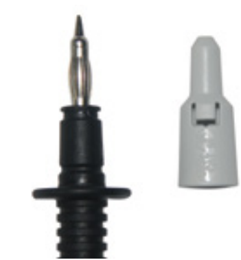
Test lines in accordance with EN-61010-031 CAT III Cap removable for CAT II environments
