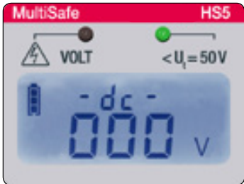
Indication of absence of voltage
