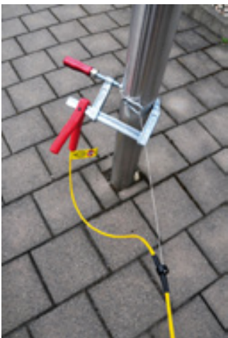
Ground connection, e.g. on the mast or with earth spike through clamp with strain relief
